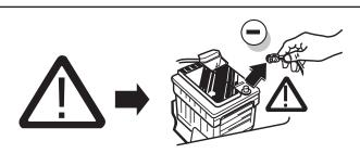
Note: It may be necessary to check if this vehicle has a stored radio code before disconnecting the battery!
